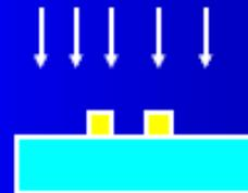
Expose wafer with UV light through mask and etch wafer
